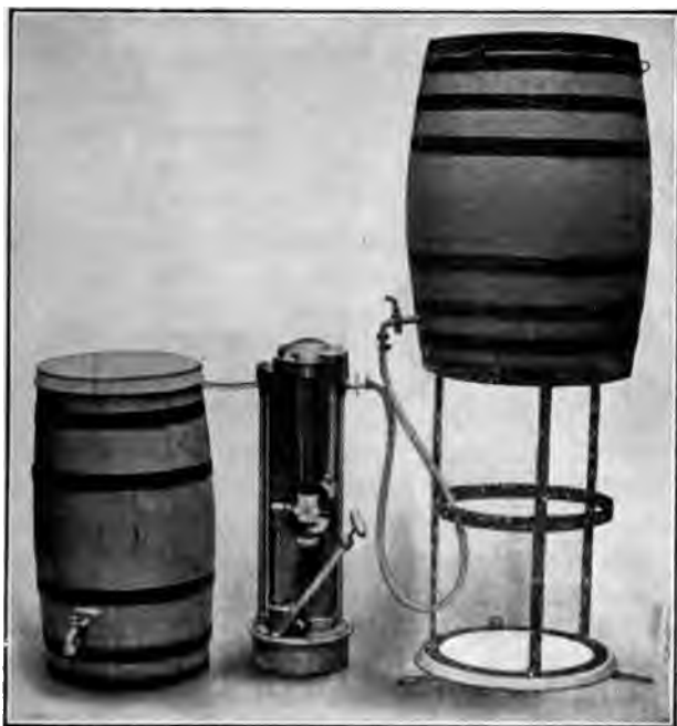
16. 46.—Barrel accessory set up, ready for operation in connection with the Forbes sterilizer.
